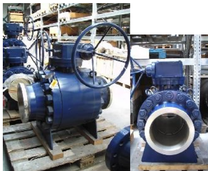
Ball valve 10" full bore 900 LBS (pallnr 2)
