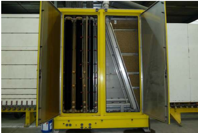
Glass Plate waschingmachine
