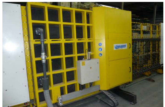
Tandem-assembly-/press robot with automatic gasfilling
