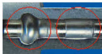
The fuel gallery of a diesel fuel injector is machined using ECM. The unique ability to precisely machine fixtures to isolate passages makes ECM a valuable tool for many industries.
